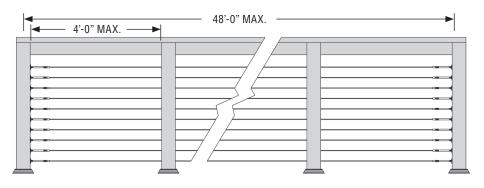
For straight cable sections using the RailEasy<sup>™</sup> Tensioner at each end, you may run cable up to 48 feet in total length (mid post required as specified).
