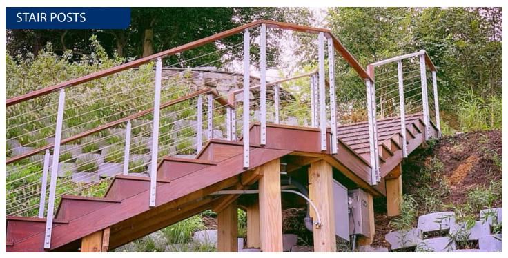
Spectrum Stair Posts are slotted on two sides to allow cable and fittings to pass through while matching the angle of the stairs. The series of posts can accommodate stair angles ranging from 26 to 43 degrees. Slots are spaced properly to meet code compliancy. Post mounting hardware is NOT included!
