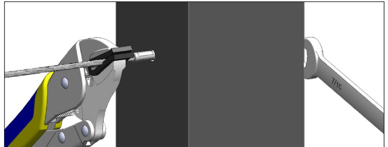
Figure G. Option two (2) is to use a cable grip pad to hold the cable just outside the post while tightening the nut.
