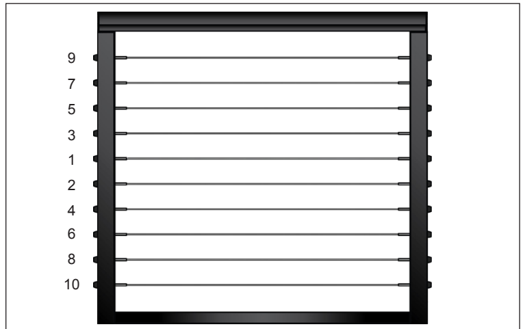
Figure H. Begin with the center run of cable and alternate working above and below until all the cables are tight.
