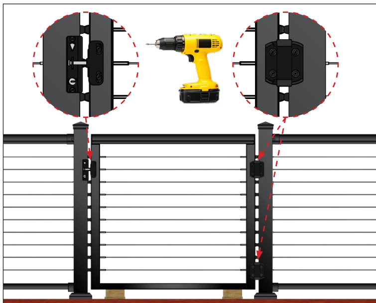
Figure L. Utilizing the NOVA II Gate locking latch and hinge hardware screw in with a #2 Phillips driver bit the supplied #10 x 1 self drilling screws.
