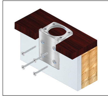
Figure M. (Left) Install four (4) 1/2" lag bolts.
